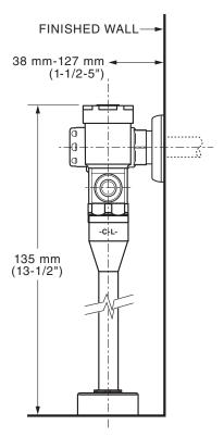
\*Note: The Critical Line (-C-L-) on Vacuum Breaker must typically be 6" (152mm) minimum above fixture. Consult Codes for details.
